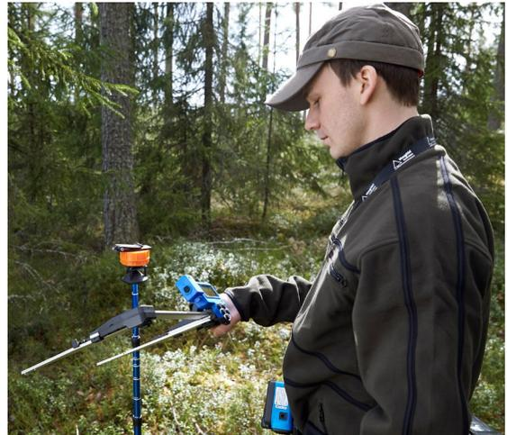
The DP GPS has a 33-channel high-sensitivity receiver that supports several satellite systems such as GPS, Glonass, Galileo and GZSS. The ability to use several satellites from
